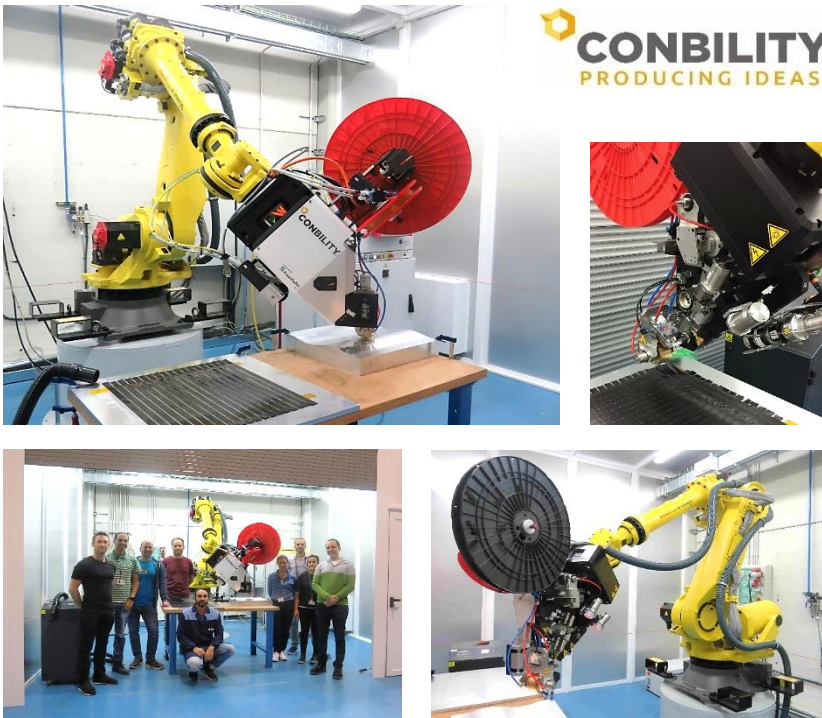
Picture 1: Tape Placement Applicator "PrePro 3D" at the Technical Center of AIMEN in Spain. Copyright: Conbility GmbH.
